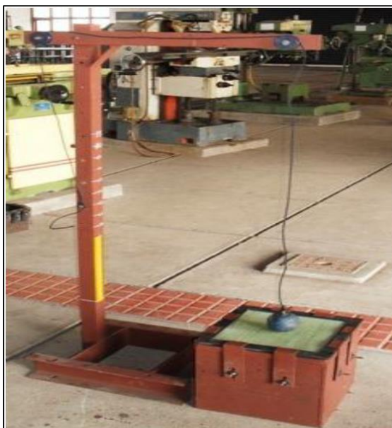
Figura 2.24 - Dispositivo de ensayo [Gayatri Vineela. M, Gayathri Tadepalli, A. Krishnaiah (2016)]
